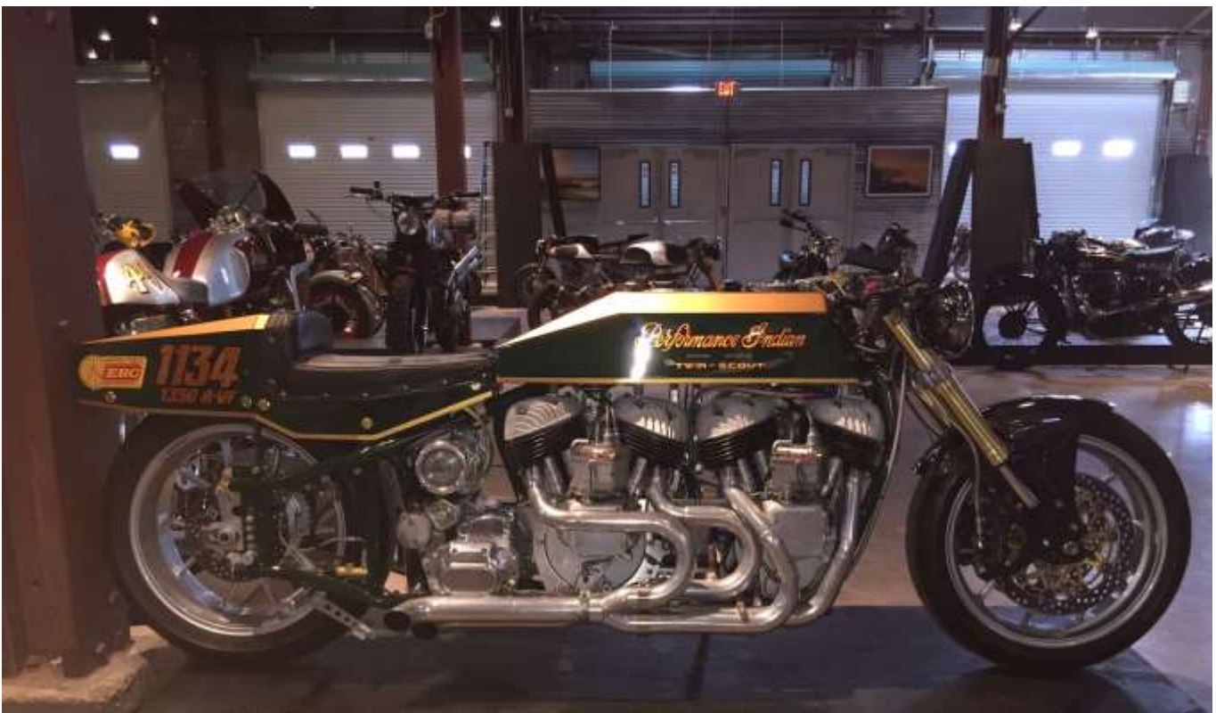
A Full Hand Built, Twin Flathead Indian Motors, Bonneville 4X World Record Holder built by Jim Mosher, Sante Fe NM.
